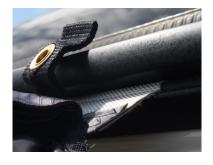
8. Take the awning piping and slide it through the awning channel, until the awning is in the desired position on the vehicle. We recommend someone else holding the flysheet up whilst you do this.
